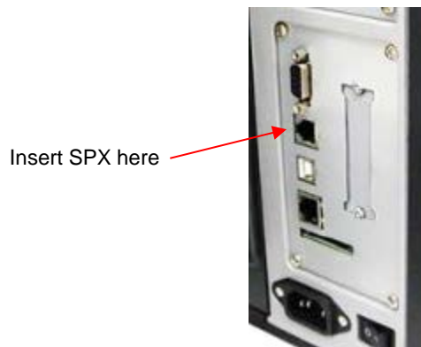
Figure 16 Inserting The SPX into the Debug Port
